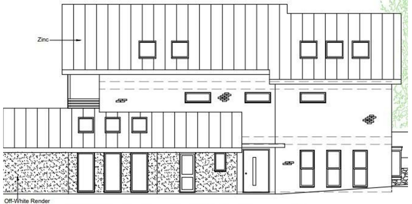
Elevation (North East) / Section AA As Proposed
